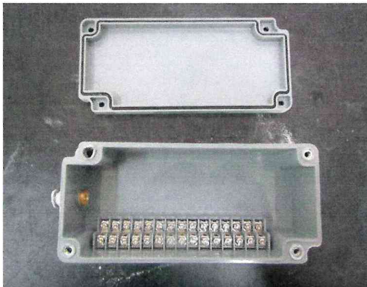
Photo 1-2 IP6X test result
