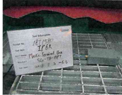
Photo 1-1 IP6X test set-up
